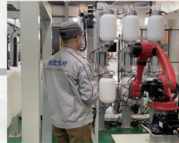
Plastic Liner Cooling and Solidification
