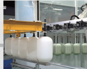
Plastic Liner Staging Buffer
